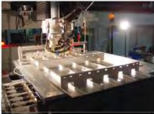
Laser beam welding process for entire panel
