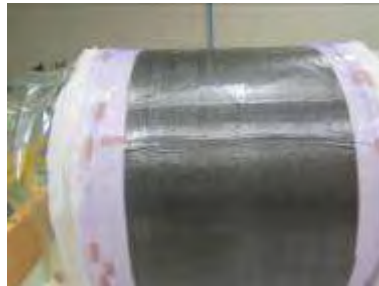
Skin lamination on auxiliary tool
